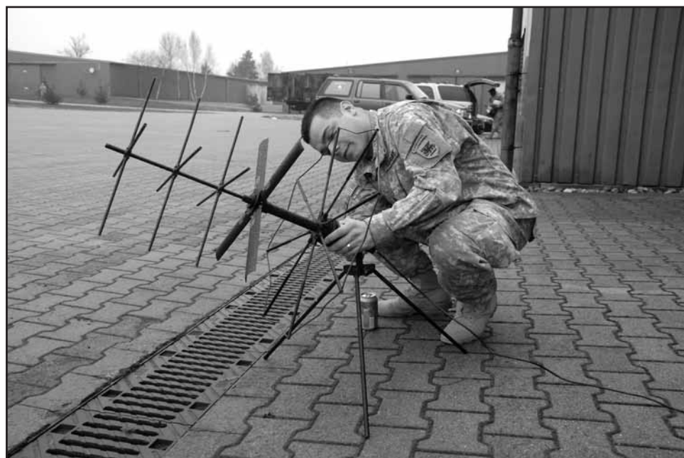
Sgt. Edwin Laboy, who works in the SETAF plans and operations section, adjusts an antenna to obtain better signal reception for the tactical satellite radio, which can be used to provide voice communication during deployments. The test was part of readying equipment in support of Task Force Recovery (Land), a joint command responsible for mitigating possible damage caused by a falling U.S. satellite.
